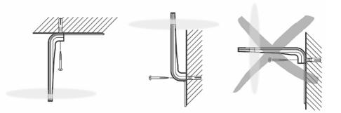
Figure 8. External antenna installation
